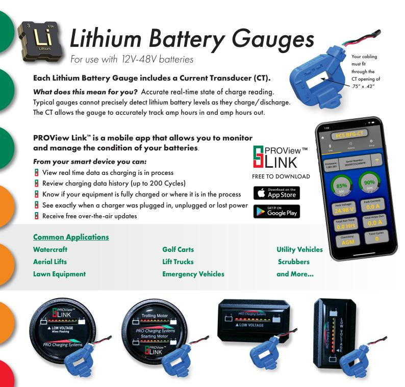
**Round Gauges** Weight: 8 oz. Size: 2.25" diameter x 2.5"L For cable length and installation details, please see our installation guide. **Rectangular Gauges** Weight: 8 oz. Size: 2.1" x 1.25" For cable length and installation details, please see our installation guide.
